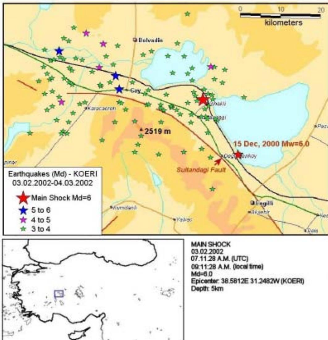
Figure 2. The main shock and the aftershock distribution
