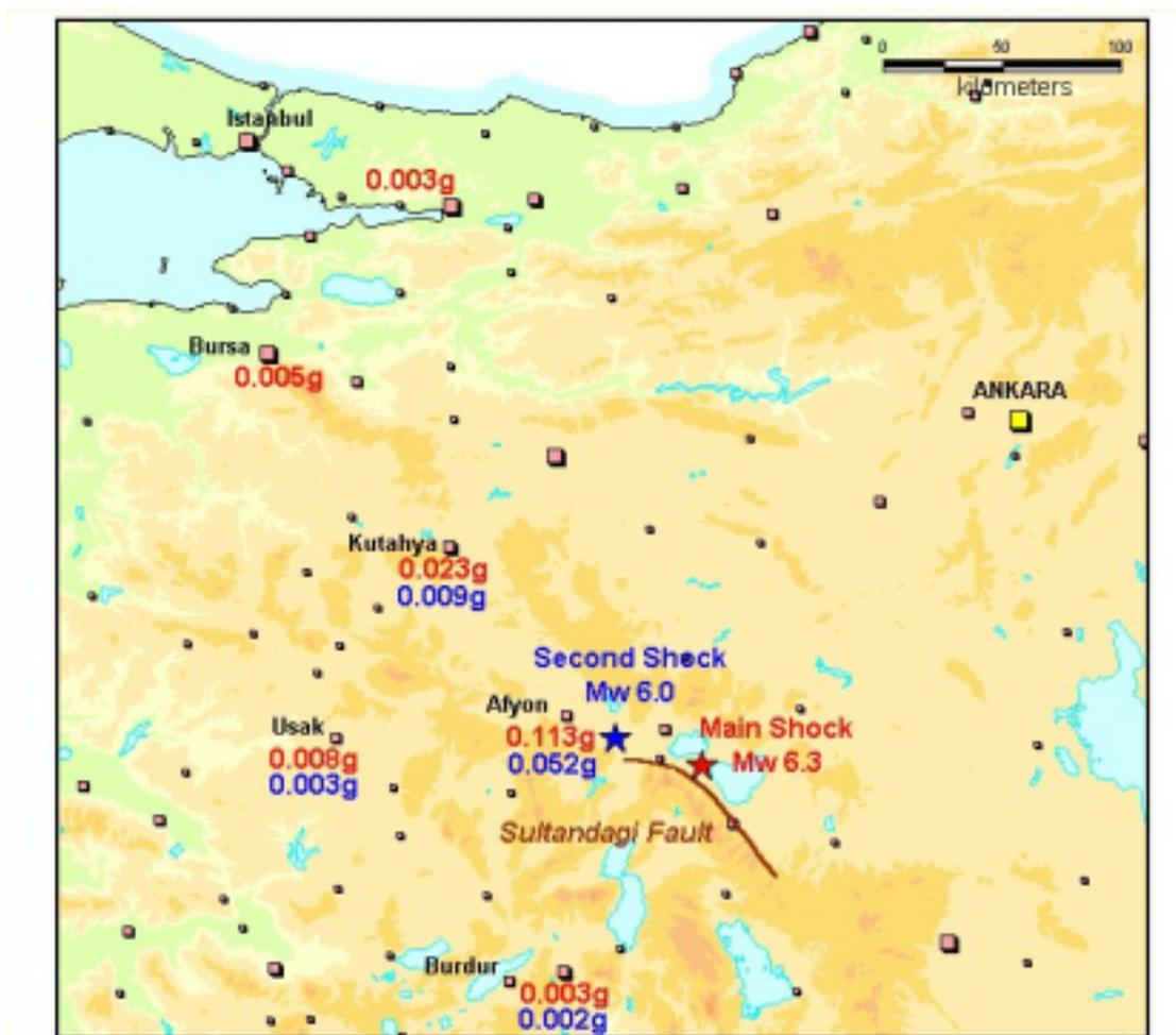
Figure 4. Peak ground accelerations recorded from the Mw=6.3 event (indicated in red) and from the Mw=6.0 event (indicated in blue).
