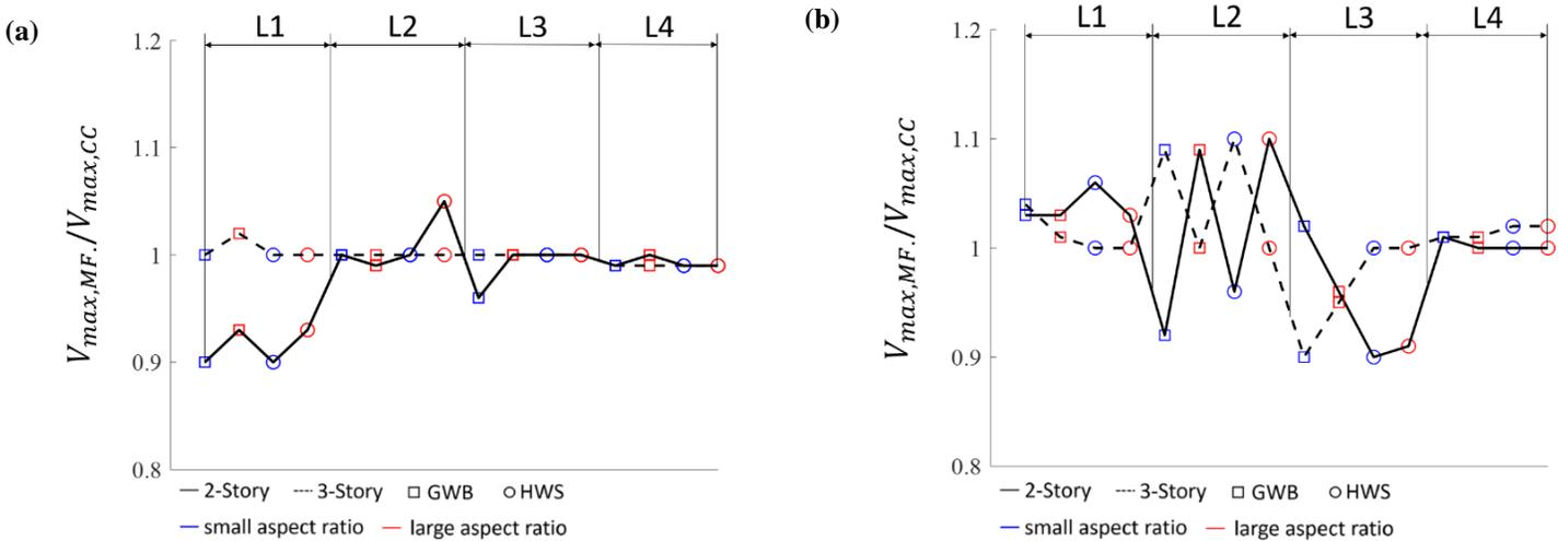
**Fig. 3** Ratio of maximum base shear from pushover response between OMF-retrofitted archetypes and SCC-retrofitted archetypes is presented for the X-direction (a) and Y-direction (b).
