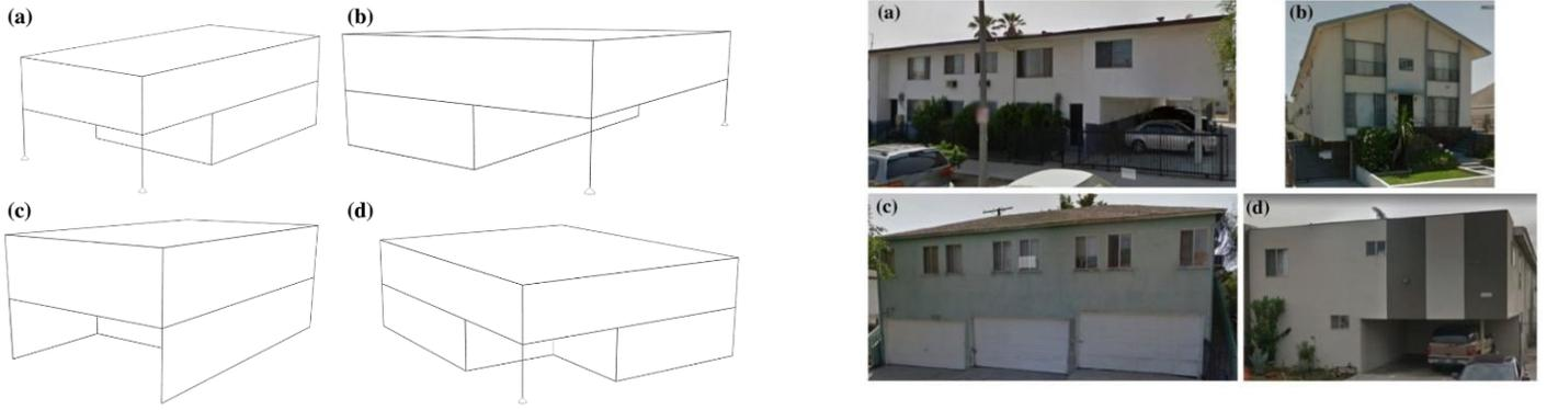
**Fig. 1** Schematic isometric views of typical SWOF woodframe building configurations (Burton et al. 2019) identified from survey (left), along with photos of typical SWOF woodframe building configurations (right): **a** L1, **b** L2, **c** L3 and **d** L4
