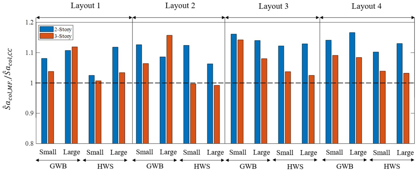
Fig 4. Ratio of median collapse capacity between OMF and SCC-retrofitted SWOF buildings.
